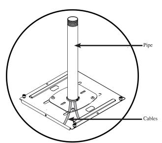
**Step 5.** At this time, run all existing cables through the pipe and down through the upper plate.
